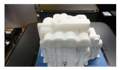
Here is the completed part prior to removing support material.
