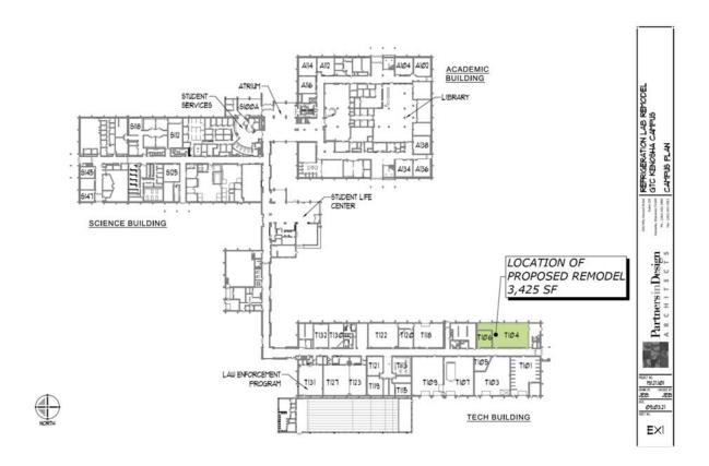
The proposed 3,425 square feet Refrigeration Lab and Classroom Remodel includes a 2,461 square feet refrigeration lab, a 614 square feet classroom with seating for eighteen students, and a 350 square feet main refrigeration rack room. The project includes a new exterior double door leading to the new condenser patio.
